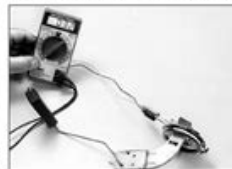
5.5 If necessary, remove the fuel level sending unit and measure the resistance while manually operating the float
