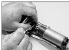
4.9 Lift tab on main electrical connector and disconnect it from the fuel pump
