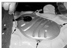
4.4 Remove screws (arrowed) from the fuel pump/fuel level sending unit access cover
