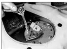
4.6 Remove the nuts that retain the fuel pump to the fuel tank
