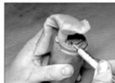
4.12 Prise off the retaining clip and detach the filter (sock) from the pump
