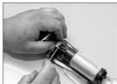
4.8 Remove the blue protective connector from the main electrical connector
